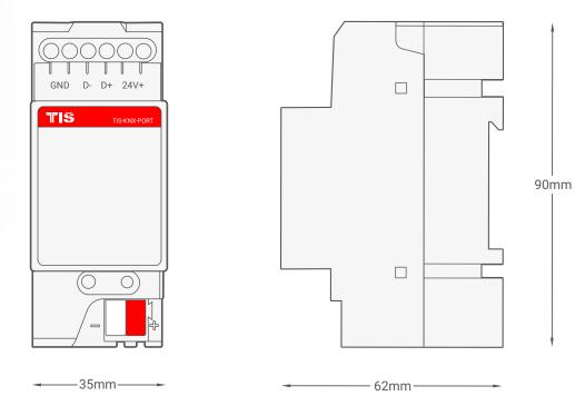
Figure 2: Module's Dimensions
